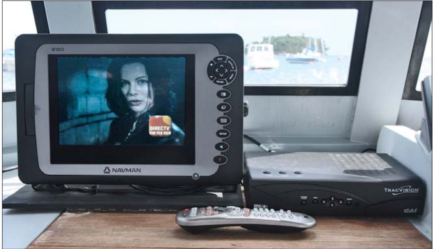
The M3 system, seen here outputting TV to a Navman 8120, includes a RF remote, and thus the purpose-built 12-volt receiver/controller, already unobtrusive, could be tucked away in a cabinet.
