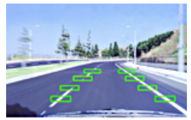
Camera-enabled system helps keep drivers in their lane.
